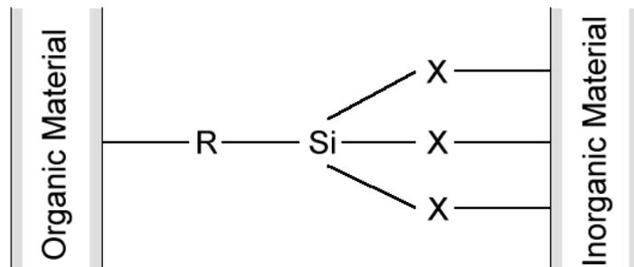
Silicone (Si) is the center of the silane molecule which contains an organic functional group (R) [ex: vinyl, amino, chloro, epoxy, mercapto, etc.], with a second functional group (X) [ex: methoxy, ethoxy, etc.]. The functional group (R) will attach to an organic resin while the functional group (X) attaches to an inorganic material or substrate to achieve a "coupling" effect.
